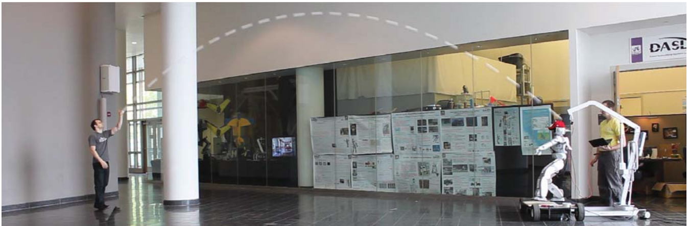
Fig. 14. Frame overlay of the Hubo throwing overhand a distance of 10 m (32.8 feet) with a release angle of 40^\circ and a tip speed of 10 \frac{m}{s} . Captured at 20 fps with a shutter speed of 1/30 sec. Each of the white dashes of in the image is the actual baseball as picked up by the video camera.
